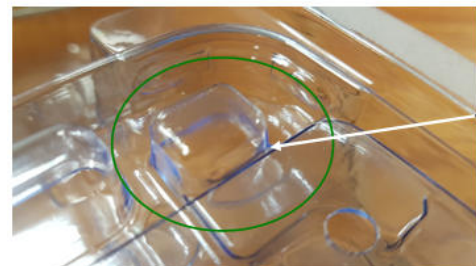
Figure 2 – PETG support plate well clipped
