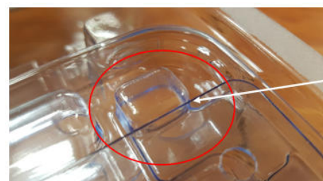
Figure 3 – PETG support plate unclipped
