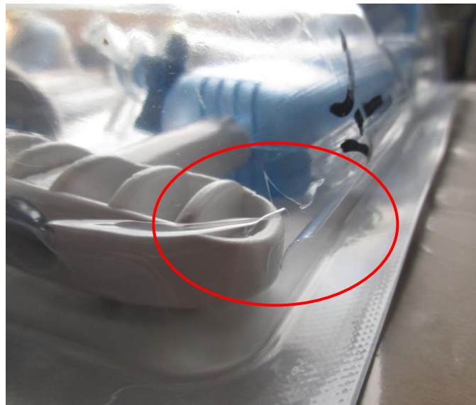
Picture 1: Example of crack observed near the inflation device handle
