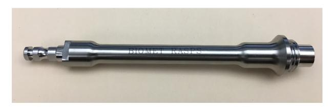
Zimmer Biomet is conducting a lot specific medical device field safety corrective action (Removal) for the Calcar Trimmer Shaft. The potential issue associated with the instrument is that the end of the shaft could fail to effectively mate with the broach.
