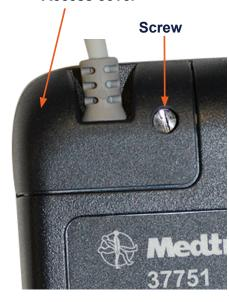
Use small Flathead screwdriver to unscrew and remove access cover.
