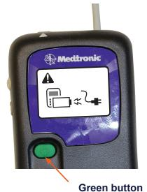
The recharger displays the AC Recharge screen. Press the green button to clear the screen.
