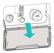
Allows patient to be manually ventilated in case of system failure (i.e. mains power and battery) or other electronic failure and is accessible behind cover on front of machine. Replaces fresh gas flow (with 100% O<sub>2</sub>) and electronic APL function.
