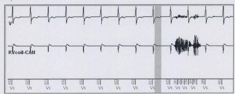
Such episodes are not related to lead malfunction. If such an episode is recurrent, avoidance of the source of interference is recommended.
