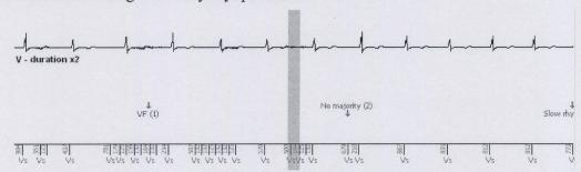
Such episodes are not related to lead malfunction. If such an episode is recurrent, sensitivity should be adjusted.
