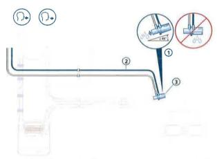
By placing the flow sensor at an angle of at least 45°, possible water condensation is prevented.
